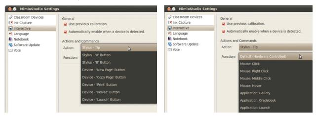
\* Seven buttons can be used with the Mimio Interactive Xi (3 stylus, 4 Xi bar). Four buttons can be used with the MimioTeach (3 stylus, 1 Teach bar)
